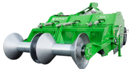
Ridge forming roller Ø178 mm
